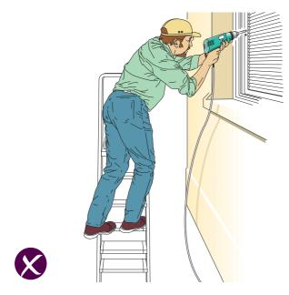
Figure 3b Incorrect - rungs side-on to work activity
