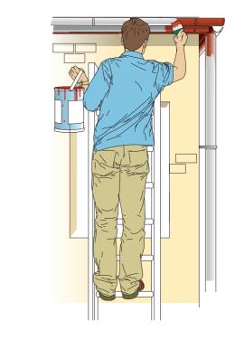
Figure 5b Incorrect - user not maintaining three points of contact
