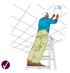
**Figure 4a** Correct - three clear steps. Dont work any higher up this type of stepladder
