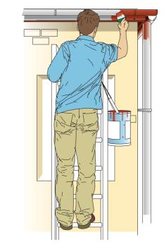
Figure 5a Correct - user maintaining three points of contact
