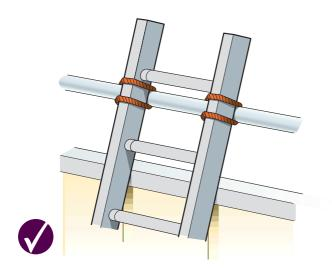
Figure 7a Correct-ladder tied at top stiles (correct for working on, not for access)
