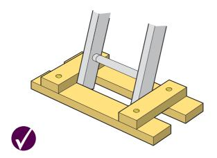
10 Do not overreach. Move the ladder so that you can keep your belt buckle (navel) inside the stiles and both feet on the same rung throughout the task. Do not place a foot on another surface, such as a window frame, to extend your reach.
