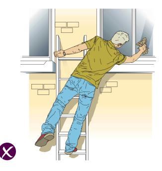
Figure 6 Incorrect - overreaching and failing to maintain three points of contact
