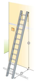
Figure 2 Ladder showing correct 1 in 4 angle (means of securing omitted for clarity)
