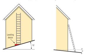
Figure 1 Ladder showing maximum angles at  $16^{\circ}$  on a slide slope and  $6^{\circ}$  on a back slope
