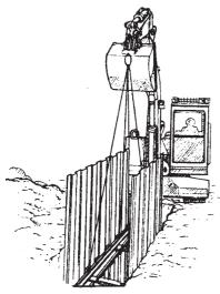
A range of proprietary trench boxes and hydraulic wallings allow trench supports to be put in place without requiring people to enter the excavation.
