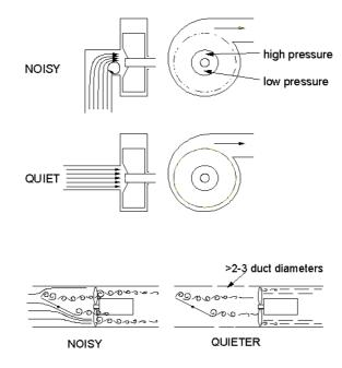
Ideally, for maximum fan efficiency and minimum noise, make sure there is at least 2 - 3 duct diameters of straight duct between any feature that may disturb the flow and the fan itself. Noise reductions of 3 - 12 dB are often possible.
