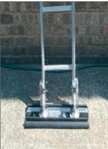
Ladder stays must be used and where practicable the ladder must be tied off to an appropriate location in order to prevent sideways movement of the ladder in either direction.
